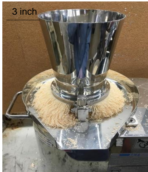
commercial basket extruder and the extrudate
