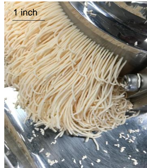
commercial basket extruder and the extrudate
